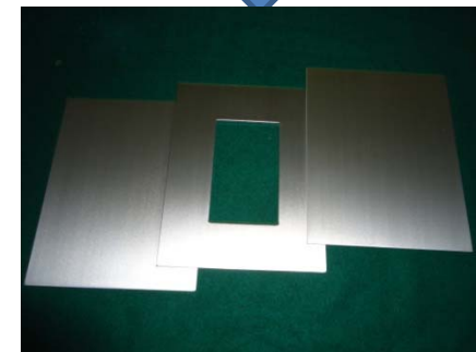
Fig. Frame, cover and fuel core of U_3Si_2/Al
