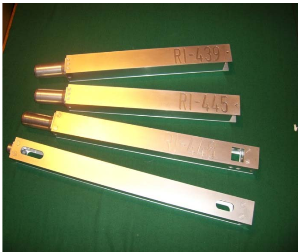
Fig. \text{U}_3\text{Si}_2/\text{Al} fuel element and control element
