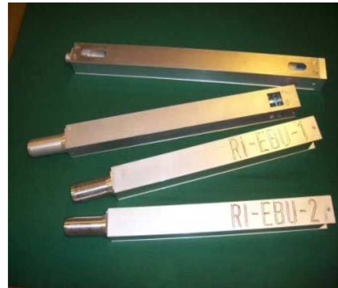
Fig. U_3Si_2/Al fuel irradiation test configuration ( stringer )
