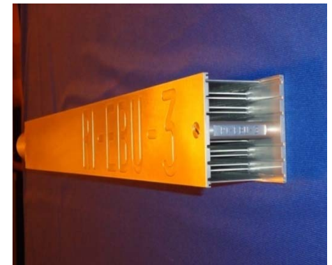
Fig. U-7Mo/Al and U-6Zr/Al irradiation test configuration ( stringer )
